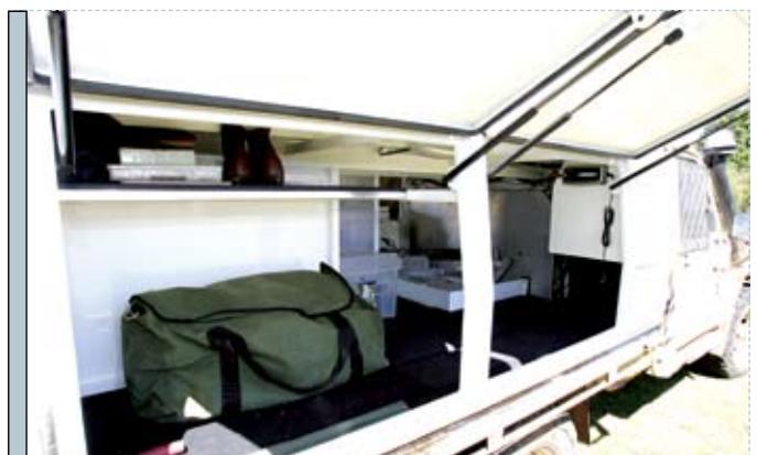
On the opposite side to the kitchen, it's almost all dust/waterproof storage space and dead easy to access through either of the two doors. Note how they give a degree of rain protection too when they're up – that's the sort of thing an all-weather camper loves
