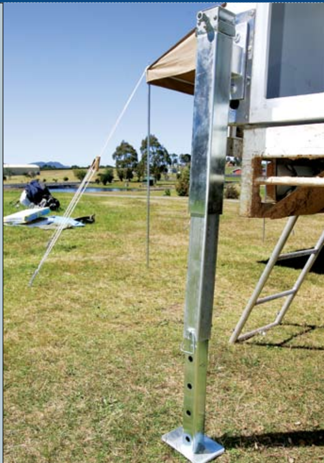
Four AL-KO corner jacks can be wound up to lift the Tray Topper off the truck, so you can leave it set up and head to town for more beer if you really have to. These are over engineered to buggery to support a mere 320kg between them
